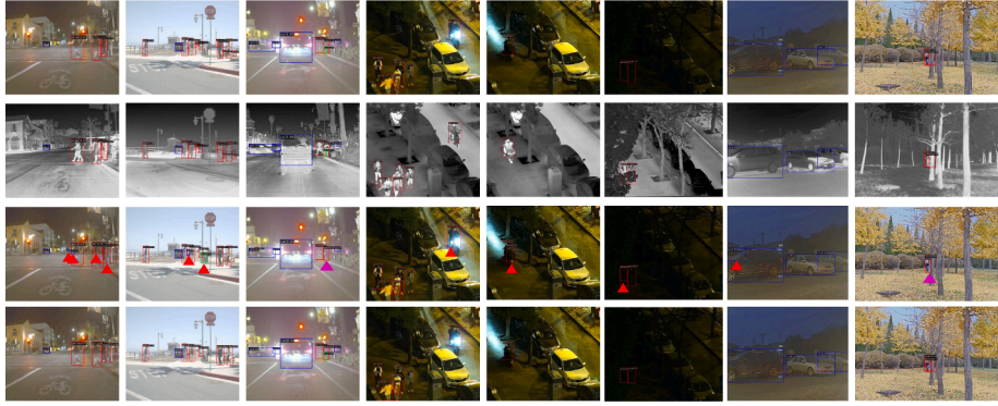
Fig. 6. Sample detections of our method on FLIR, LLVIP, and M 3 FD datasets. The first and second rows are the input RGB and IR images, the third row is the detection result of the baseline, and the fourth row is the detection result of our method. The red triangle markers indicate false detections of the baseline, while the pink triangle markers indicate missed detections of the baseline. (For interpretation of the references to colour in this figure legend, the reader is referred to the web version of this article.)
