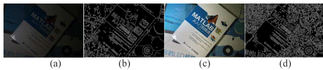
Fig. 10. Edge detection results of images before and after enhancement. (a) is the original image; (b) is the edge detection on (a); (c) is the Enhanced image of (a); (d) is the edge detection on (c).
