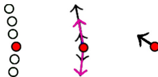
Fig. 2 The local structure descriptor of a point (depicted as the solid red circle) is computed from its neighbors (depicted as circles). Vectors originating from the point to their neighbors (shown in the middle) are summed to get the local structure descriptor
