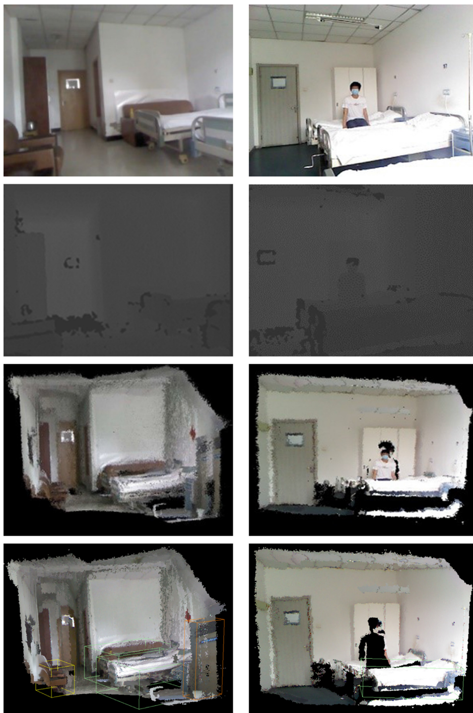
Fig. 6. Examples of semantic maps. From top to bottom, the panels on each row depict the RGB image, the depth image, the rendered point cloud with color, and the semantic map. The left column shows a case with only stationary objects and the right column shows a case with non-stationary objects, in which the non-stationary objects are removed.
