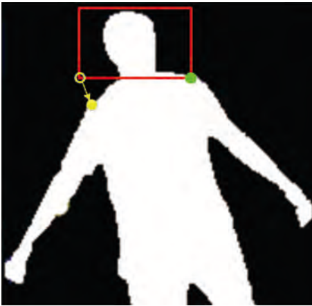
Fig. 4. Detection of shoulders. The green dot marks the left shoulder. The yellow circle marks the proposed location of the right shoulder. However, since the proposed location is in the background, a nearest foreground point is identified as the proposed location of the right shoulder, as depicted by yellow dot.
