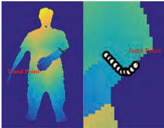
Fig. 7. An example of a searching pattern for an elbow point under self-occlusion situation.
