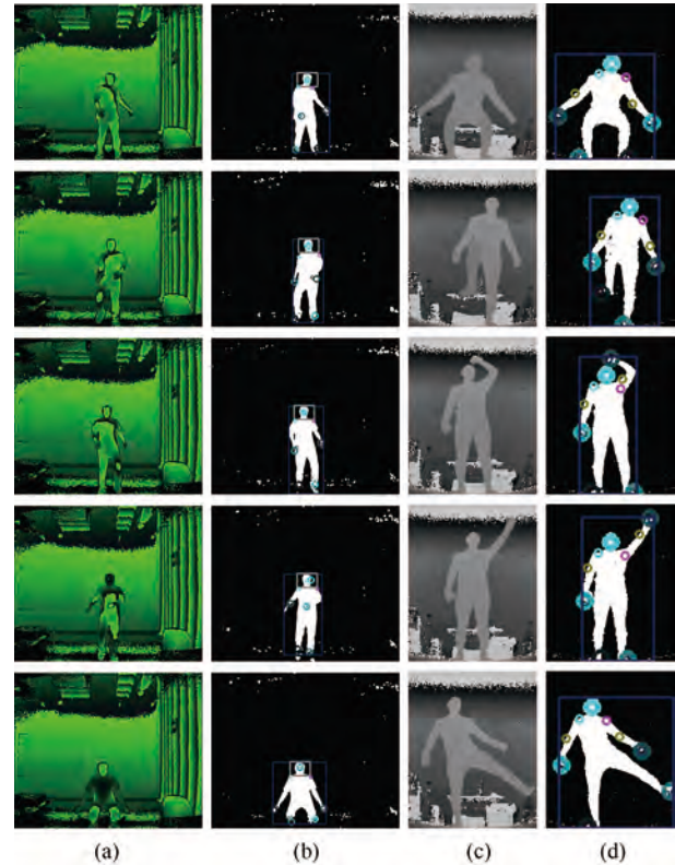
Fig. 9. Exemplar frames and the results from our method. Column (a) shows the frames from the videos of our collection and column (b) shows the results of the detected feature points. Column (c) shows the frames from the videos of SMMC-10 and column (d) shows the results of the detected feature points.
