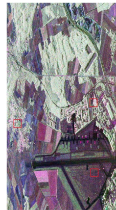
Fig. 17. ESAR image of Oberpfaffenhofen in PauliRGB. The top left box represents samples of housing area in Fig. 19(a)–(d). The bottom right box represents samples of a double-bounce reflector in Fig. 19(e)–(h). The top right box represents samples of parking lot with rows of cars in Fig. 19(i)–(l).
