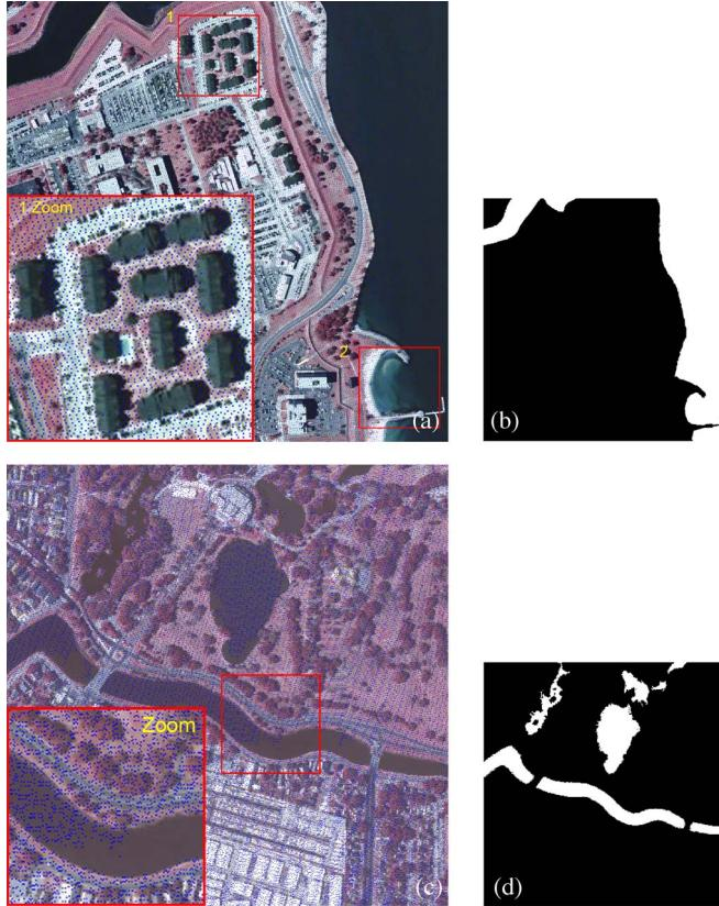
Fig. 3. Exemplar delineation results. (a) and (c) the superimposed ALSM data on images. (b) and (d) the segmentation results.
