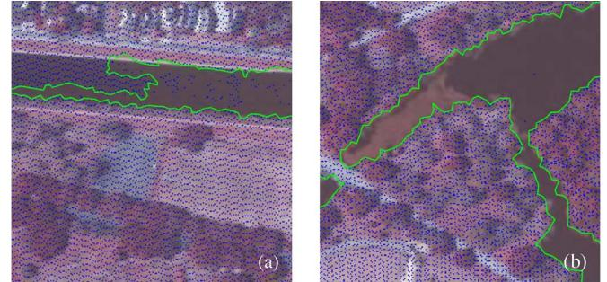
Fig. 1. Superimposed ALSM data on imagery. The contours show manual delineation of water body from ALSM data. (a) Discrepancy in different modalities. (b) ALSM measures of water body are absence.
